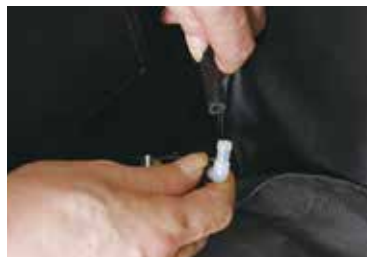
Connect air tube of armrest.
