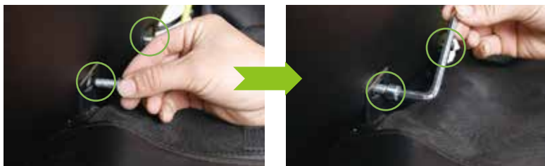
Fasten the armrest with two screws.
