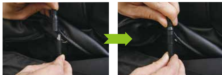
Connect back cushion heat wire.
